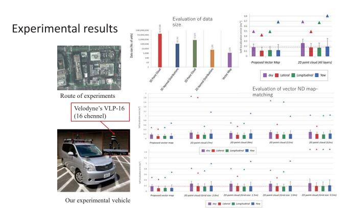
Evaluation of multilayer 2D vector structure (comparison with conventional 2D methods)
