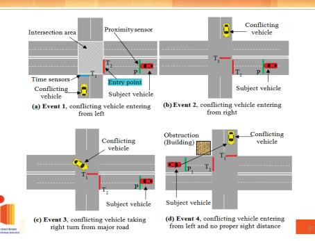
FIGURE 3Sketch of simulator experiment with different events.
