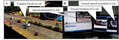
(A) Data collection and (B) Extraction process for validating speed data with different views from camera synchronized
